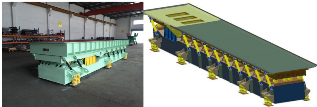
Several Options are available. For example wear plates in different materials, hood with connection for dust deducting, special trough for many different functions. Our two-mass system eliminates 98 % of all vibrations. To deliver the best technology, we produce our own drive system (Eccentric Drive HSA).
